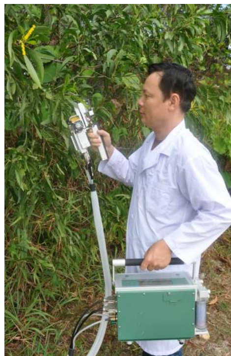
Dr Le Quang Vuong carrying out gas exchange measurement on Acacia sp. using a portable Infra Red Gas Analyzer (IRGA)
