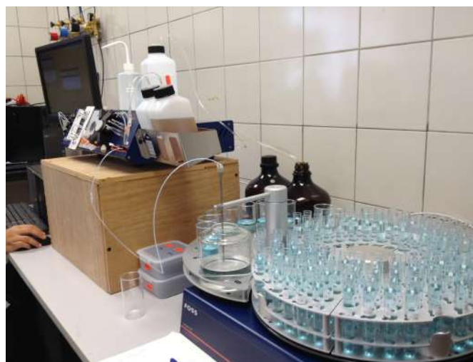
Determining Total N and P concentrations using a Flow-Injector Analyser
