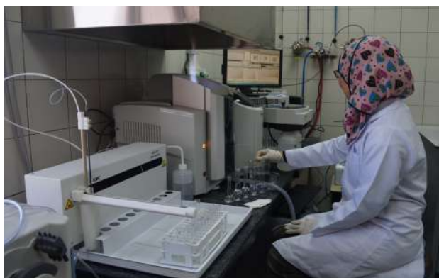
Measuring Al and macronutrient elements in acid-digested leaf and soil samples using an Atomic Absorption Spectrophotometer
