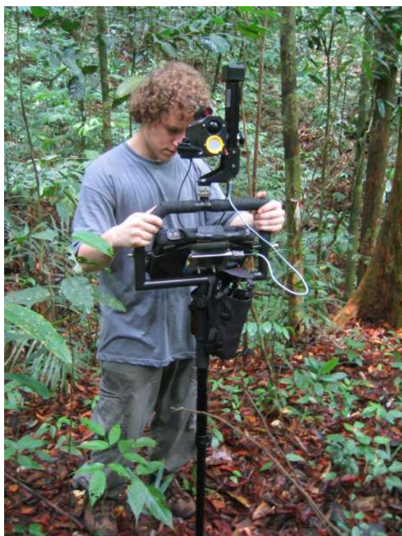
Martin Svatek using the FieldMap hardware to plot the trees
